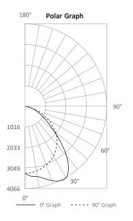
$<sup>^*\,</sup>$  80-90° glare zone is calculated by dividing the lumens in that zone by the lumen total in the 0-90° zone
