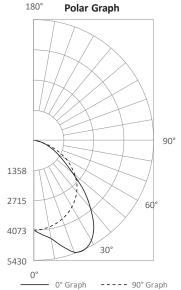
$^{\ast}\,$  80-90° glare zone is calculated by dividing the lumens in that zone by the lumen total in the 0-90° zone
